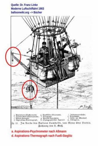
The picture shows again the drawing with the basket of the gas balloon Humboldt and its instruments. The aspirated psychrometer and the aspiration thermograph are encircled red. Both are right beyond the basket, so that the measurements take place beyond the area by the temperature of the basket influenced air. Namely the aspirated psychrometer in a rack on eye level to be able to read it during the journey with the help of binoculars. And the aspiration thermograph hangs below the basket.
