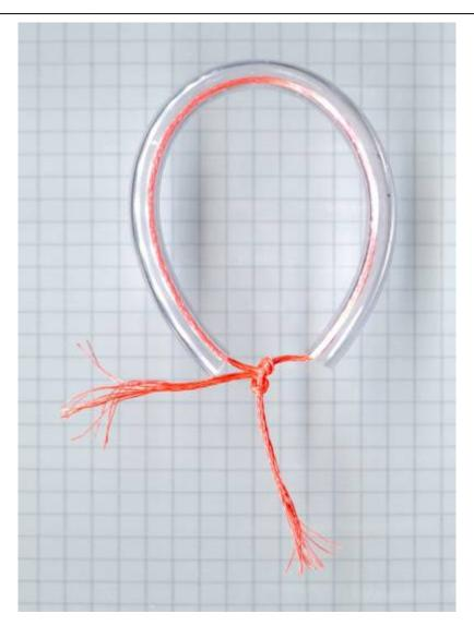
Then the tube is pulled together with the thread to form a balloon shape, and then the thread is knotted.
