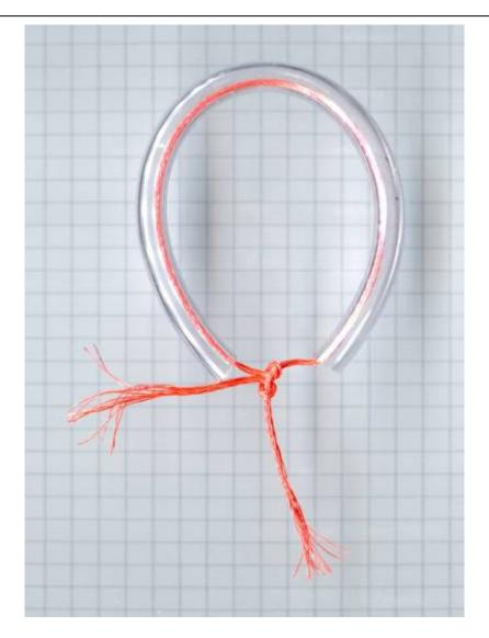
Then the tube is pulled together with the thread to form a balloon shape, and then the thread is knotted.
