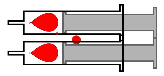
In the schematic drawing above, the tap is open, air can flow in and out of the syringe unhindered. The air pressure inside and outside the syringe is the same.
